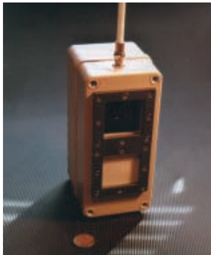
A portable, radio-linked PIR/CCTV unit. Although much larger than the miniature printed circuit board, this unit has the advantage that it needs no wiring – an invaluable asset where some historic fabric is concerned. (Edgarsson Security Designs)
